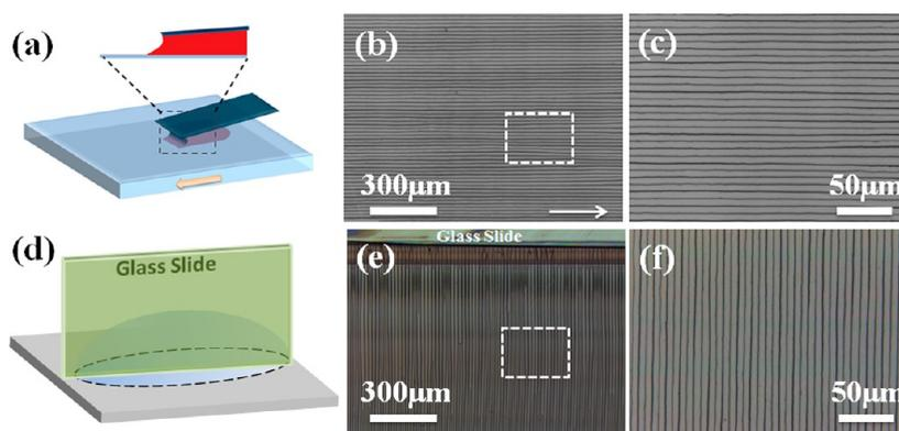
**Figure 4.** Constrained evaporation in the confined geometries composed of (a) two nearly parallel plates, and (d) a slide situated vertically to a rigid substrate rendered the controllable formation of regularly spaced parallel microchannels. (b and c) Optical micrographs of periodic microchannels formed from (a). (e and f) Optical micrographs of periodic microchannels formed from (d).
