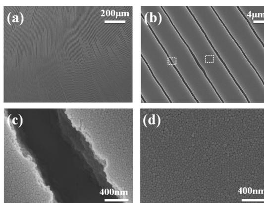
**Figure 2.** (a and b) Typical SEM images of microchannels (*i.e.*, cracks) formed on the Si substrate at different magnifications. The left and right dashed boxes in panel b correspond to the close-up images in panels c and d, respectively. (c) SEM image showing that the edge of cracks was very sharp. (d) SEM image of closely packed PS nanoparticles on the surface of microscopic PS patterns.
