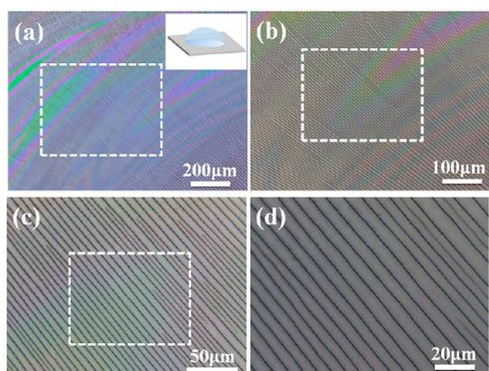
**Figure 1.** Optical micrographs of highly ordered spoke-like microchannels on the Si substrate at different magnifications. The dashed boxes in panels a, b, and c correspond to the close-up optical micrographs in panels b, c, and d, respectively. A schematic representation of drying PS nanoparticle suspension on a Si substrate is shown as an inset in panel a.
