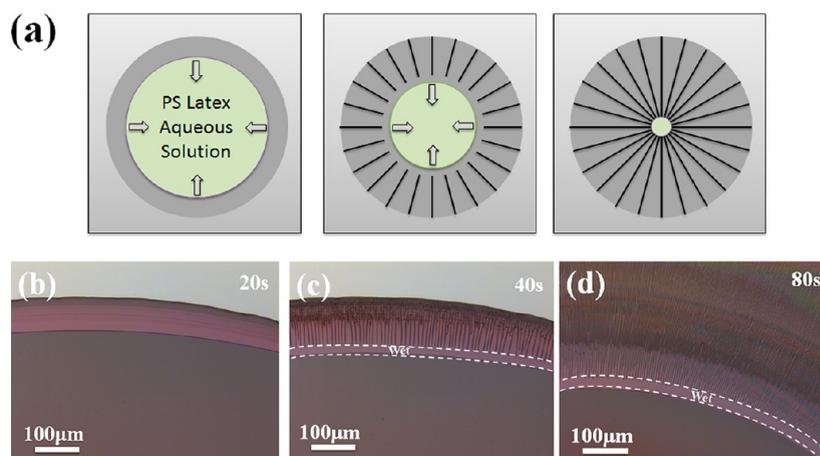
**Figure 3.** (a) Schematic stepwise representation of the formation of microchannels (*i.e.*, cracks) via drying-mediated self-assembly of highly concentrated PS nanoparticle suspension. (b–d) Optical micrographs of drying front taken at different times ((b) 20 s, (c) 40 s and (d) 80 s) from the *in situ* optical microscopy measurement. The wet region was marked (*i.e.*, “wet”) within two dashed curves in panels c and d.
