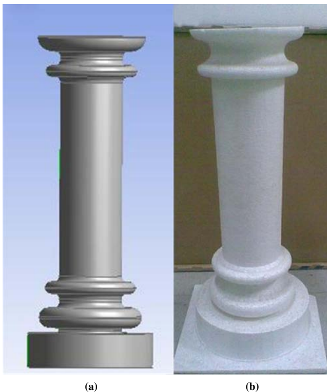
Figure 14 CAD model and prototype of a Roman column model
