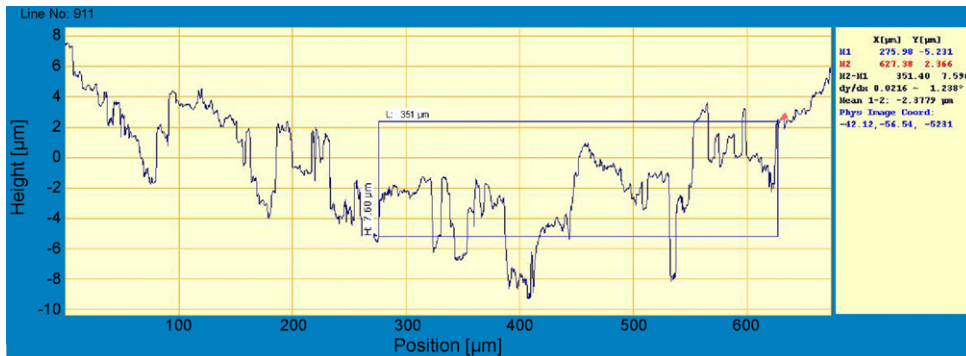
Fig. 15. Experimental worn surface profile of AISI1080 steel.
